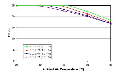
Figure 5: Maximum output power derating curves vs. ambient air temperature for airflow rates of 100 LFM through 400 LFM with air flowing from from input to output (nominal input voltage).
