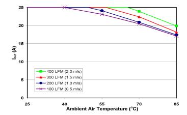
Figure 3: Maximum output power derating curves vs. ambient air temperature for airflow rates of 100 LFM through 400 LFM with air flowing across the converter from pin 1 to pin 3 (nominal input voltage).
