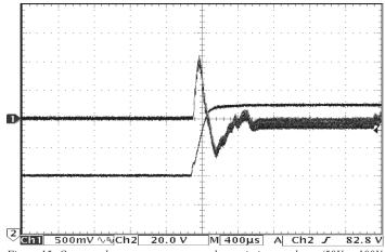
Figure 15: Output voltage response to step-change in input voltage (50V to 100V in 200 $\mu$ s). Load cap: 470 $\mu$ F, 15 m $\Omega$  ESR tantalum capacitor. Ch 1: Vout (500mV/ div), Ch 2: Vin (20V/div), at zero load current.
