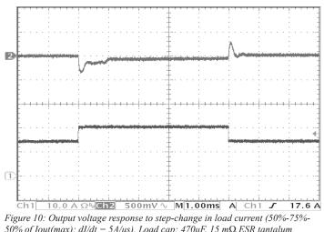
50% of Iout(max):  $dI/dt = 5A/\mu s$ ). Load cap:  $470\mu F$ ,  $15 \text{ m}\Omega \text{ ESR}$  tantalum capacitor. Top trace: Vout (500mV/div), Bottom trace: Iout (10A/div).
