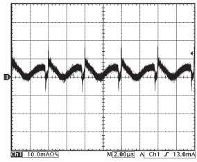
Figure 13: Input reflected ripple current, is, through a  $4.7\mu$ H source inductor, using a  $100\mu$ F input capacitor, at nominal input voltage and rated load current (10 mA/div). See Figure 11.
