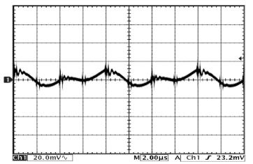
Figure 14: Output voltage ripple at nominal input voltage and rated load current (20 mV/div). Load capacitance:  $1\mu$ F ceramic capacitor and  $10\mu$ F tantalum capacitor. Bandwidth: 500 MHz. See Figure 11.
