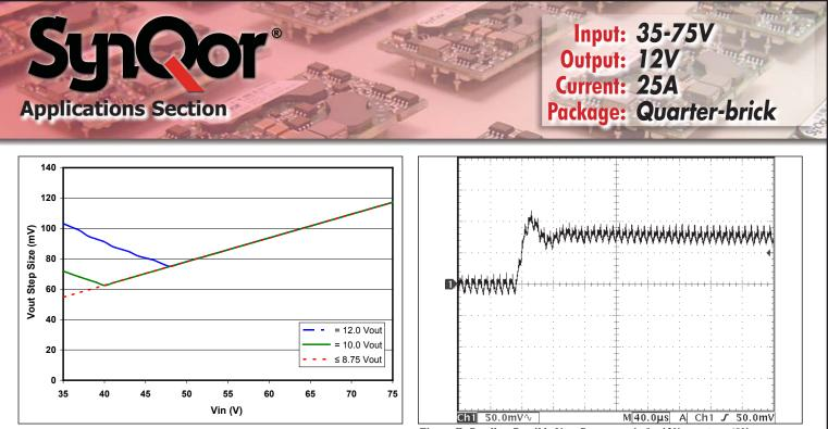
Figure E: Output Voltage Resolution example for 12Vout units.
