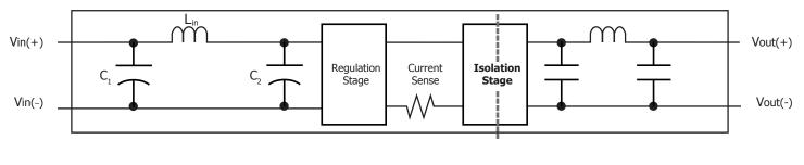
Figure D: Internal Input and Output Filter Diagram (component values listed in Electrical Characteristics section).
